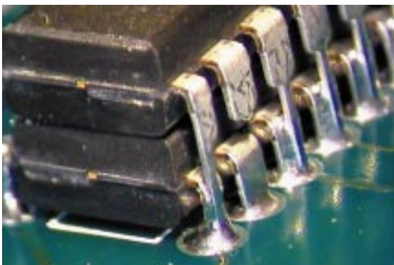
Figure 5 DIP component stacked and soldered onto another DIP component. One lead shown clipped. Note: Leads of added component should not be inserted into the plated holes.
