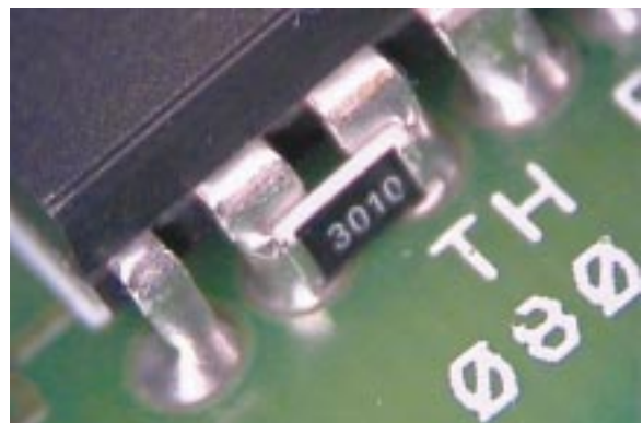
Figure 6 Chip cap bridging adjacent leads.
